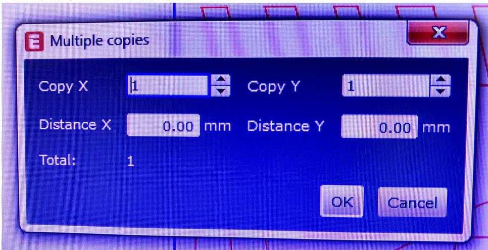
Use your measurements in the Distance X and Y axis to determine the gap between the cuts.
