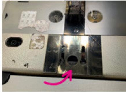
**2.** Insert the screw at the back of the guide into the hole and slide upwards
