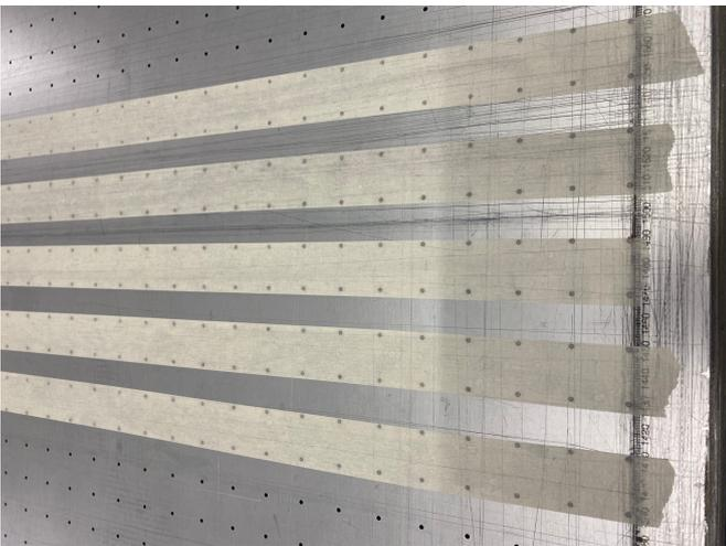
We also use masking tape to help the board stay flat on the bed.
