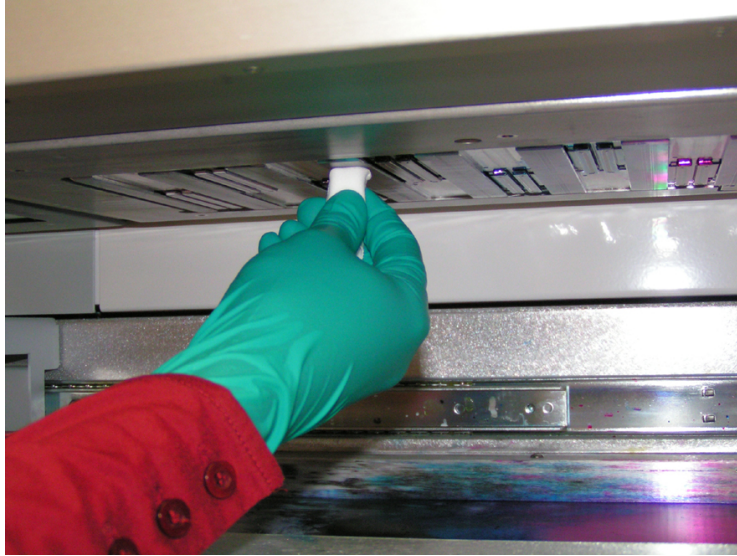
[121] Clean the nozzle plates between printheads
