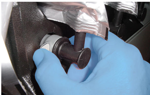
[119] Remove the Quick-Release Coupler
