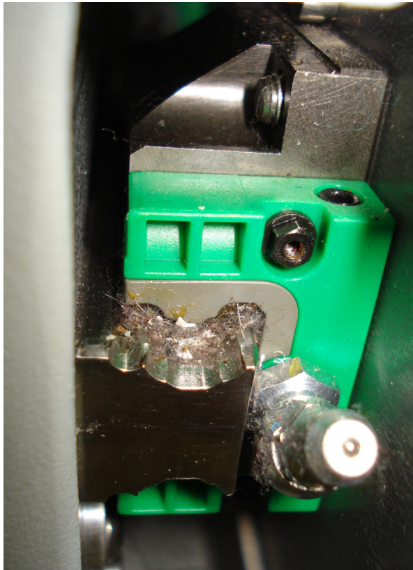
[134] Dust on the runner bearing block shields
