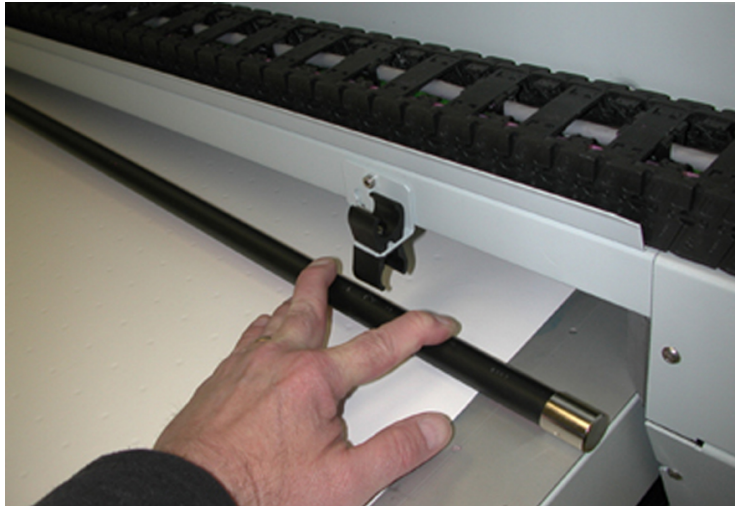
[78] Remove Static Bar
