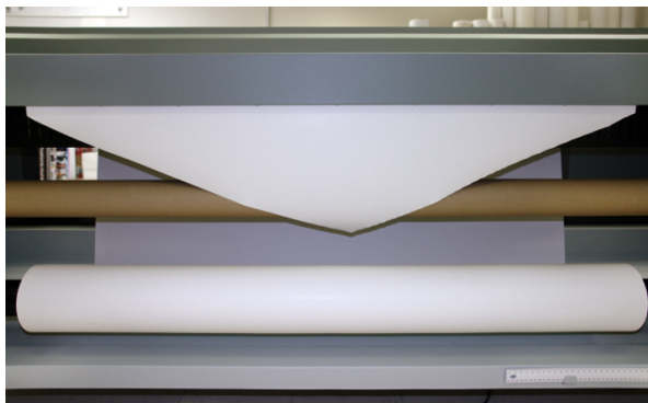
[67] Cut the media at an angle
