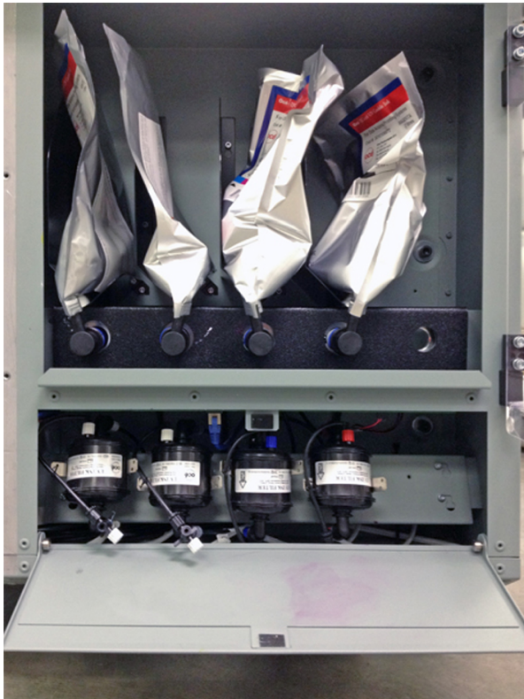
[137] Open Ink Filter Enclosure Cover
